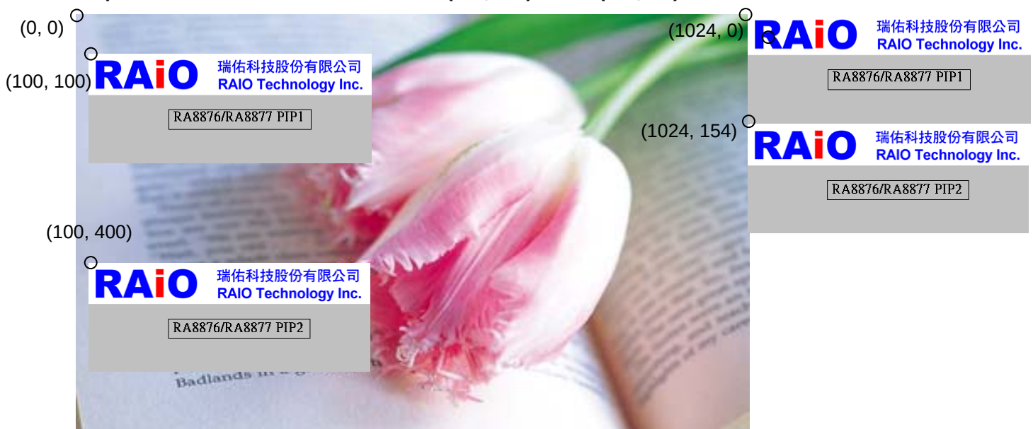
Figure 5-4 : Enable PIP and PIP 2
